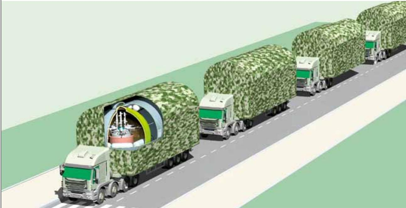
*Transportable power unit with ATGOR gas-cooled reactor*
